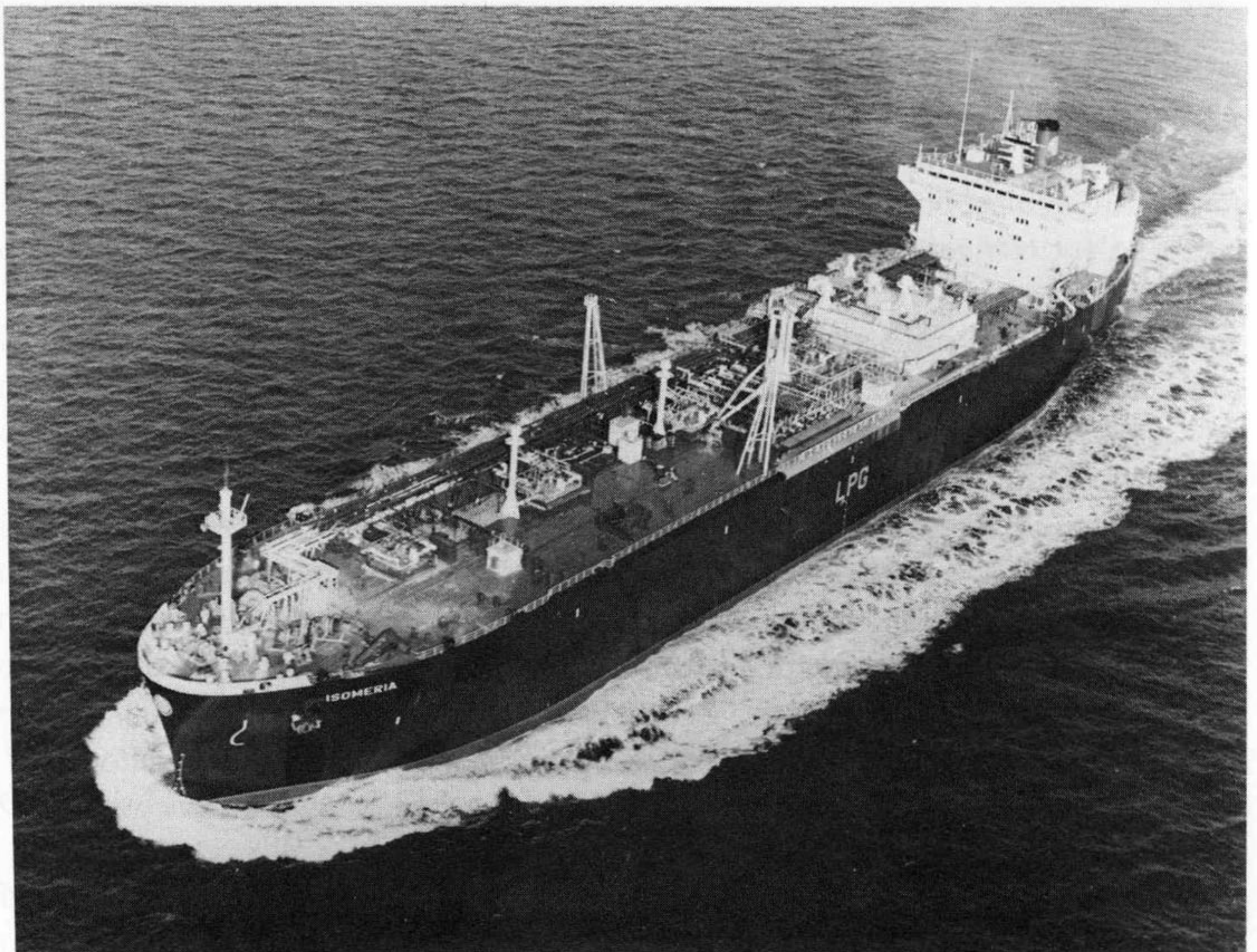
Figure 7.6 m.s. Isomeria ; 58,950 m 3 ; built 1982 by Harland and Wolff. An LPG carrier.
