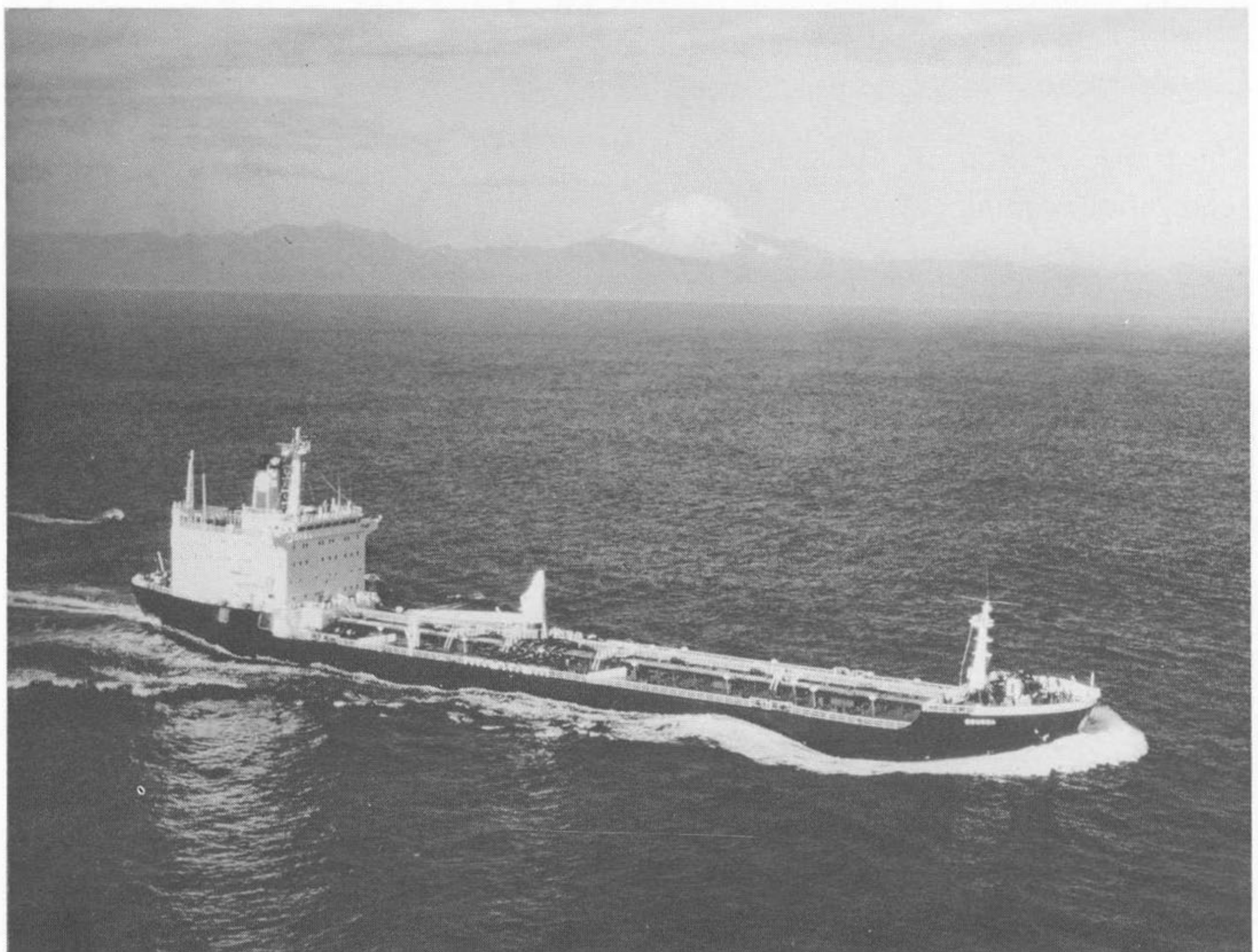
Figure 7.5 m.s. Eburna ; 31,374 dwt. A typical 1979-built products carrier, capable of carrying different grades on the same voyage. Mt. Fuji in the background.
