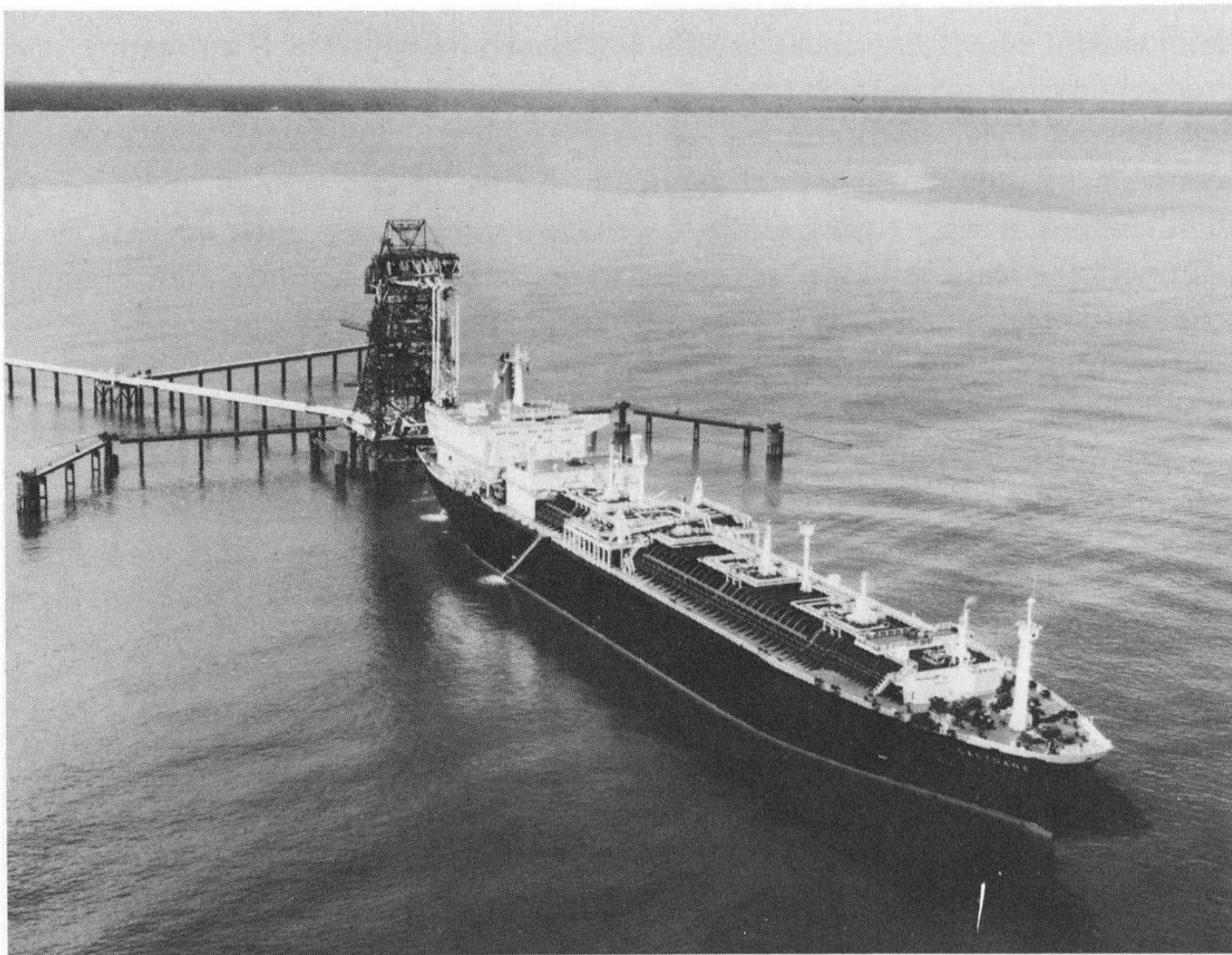
Figure 7.7 s.s. Gastrana ; 75,000 m 3 ; built 1974. An LNG carrier dedicated to the “closed loop” Brunei–Japan.
