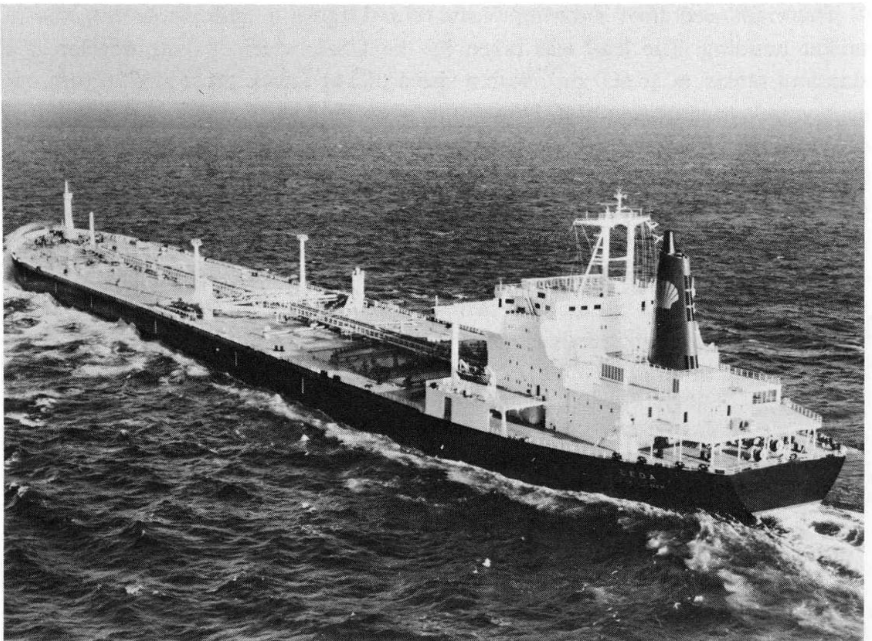
Figure 7.3 s.s. Leda ; 276,860 dwt; built 1973. An example of a VLCC, developed in response to the closure of the Suez Canal.
